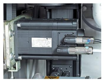
Servo-drive with positioning controller
